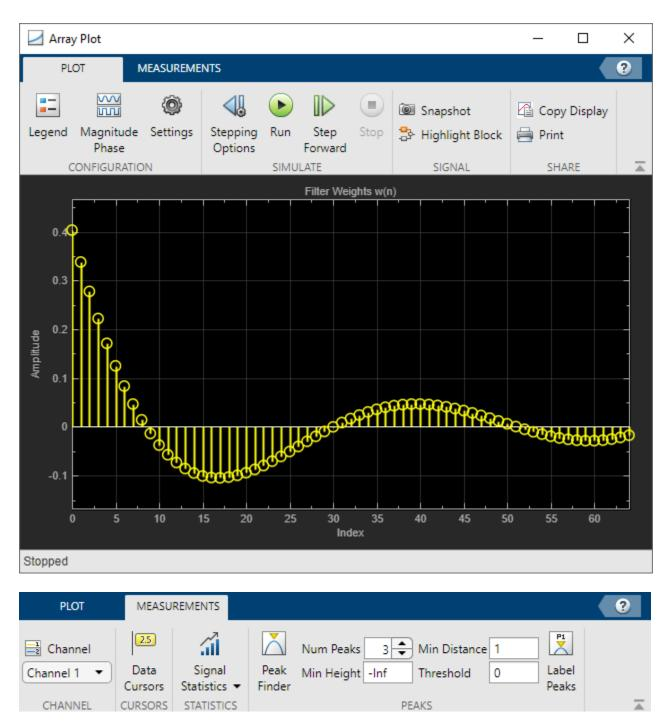
From the toolstrip, you can run the model, modify the settings, turn on measurements, and share an image of the plot.
