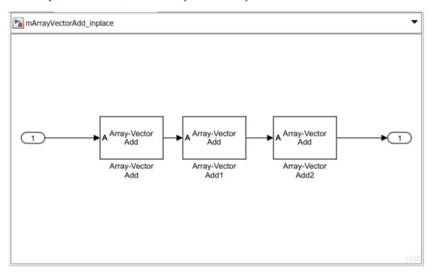
Each block adds a vector to its input data and generates an output that is of the same size as the input.
